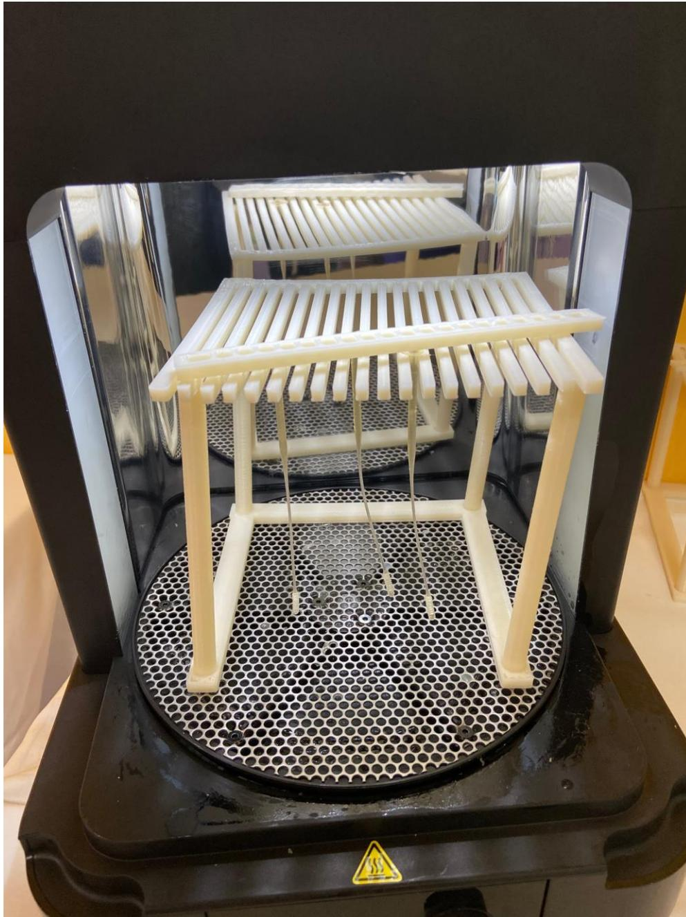
Rack made out of ABS in order to withstand the curing temperatures.
